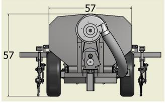
Low profile and compact size for narrower rows —57 inch overall height and 57 inch hopper width
