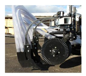
Hydraulic toolbar extensions allow the operator to adjust the toolbar width from 96 inches to 156 inches \*
